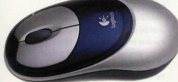
a flat surface, the ball inside rolls against small rollers that electronically determine the X or Y direction as you move the mouse. Manufacturers have even devised mouse pads in all shapes and colors to allow the roller ball to rotate smoothly. For years this simple concept has worked well, and a great many computers today still use this type of mechanical pointing device.
